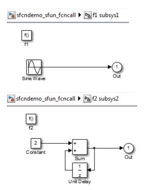
When the Pulse Generator emits its upper value, the function-call subsystem connected to the first element of the first S-function output port is triggered. Similarly, when the Pulse Generator emits its lower value, the function-call subsystem connected to the second element is triggered. The simulation output is shown on the following Scope.
