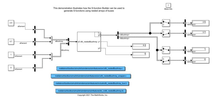
In the C code in S-Function builder, the output y0 is the nested array of buses. The output y1 is the sum of the elements of the first array of buses, aBusArray. The elements of aBusArray are aBusArray[0].aElement and aBusArray[1].aElement. The output y2 is the product of the elements of the second array of buses, bBusArray. The elements of bBusArray are bBusArray[0].bElement and bBusArray[1].bElement.
