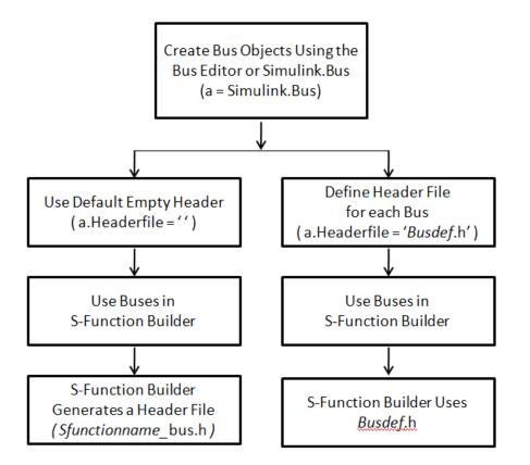
For a demonstration on how to use the S-Function Builder with a bus, enter the following command at the MATLAB Command Window:
