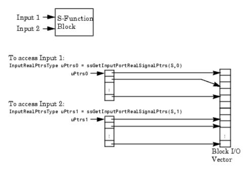
As shown in the previous figure, the input array pointers can point at noncontiguous places in memory.
