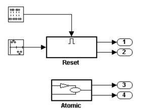
The model contains two nonvirtual subsystems, the conditionally executed enabled subsystem named Reset and the atomic subsystem named Atomic. Each subsystem contains an S-Function block that calls the S-function dsfunc.c, which models a discrete state-space system with two states. The enabled subsystem Reset resets the state values when the subsystem is enabled, and the output values when the subsystem is disabled.
